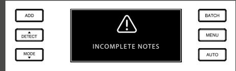
Incomplete or damaged banknote. Can occur when a torn banknote is fed through the machine. Remove and check the banknote and press **START** to continue.
