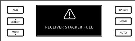
The maximum stacker capacity is 220 banknotes. Remove the banknotes from the stacker.
