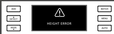
A banknote with a different height has been detected. Remove the different banknote denomination, remove the counted notes and re-count the bundle.
