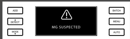
Counterfeit or suspicious banknote. MG features not detected. Remove the banknote from the stacker and press **START** to continue (Safescan 2650 only).
