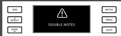
Sometimes banknotes are stuck or folded together. Check the banknotes and re-count. If this error message occurs frequently, adjust the hopper adjustment wheel slightly (+).
