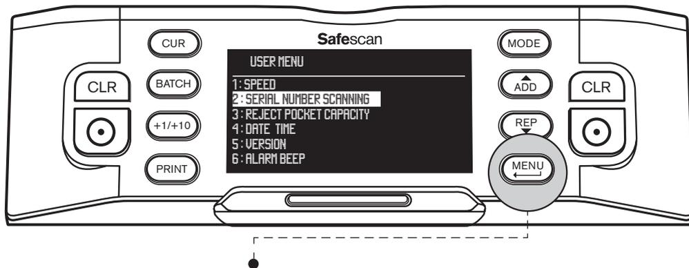
To enable serial number scanning: Press **[MENU]** to access the user menu.
