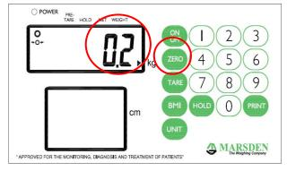
If for some reason the scale shows a reading other than 0.0kg then it can be reset to zero (2% of capacity).
