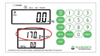
The display will show the last height entered and the extreme left digit will flash. Enter the height by using the numeric key pad (e.g. 170.0cm). There will always be an active flashing digit in the height display (unless the HOLD key is pressed).
