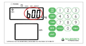
After a few seconds the scale will lock on the person's weight, the person can now stand off the scale and the weight will remain.
