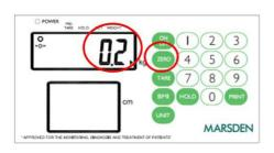
If for some reason the scale shows a reading other than 0.0kg then it can be reset to zero (2% of capacity).
